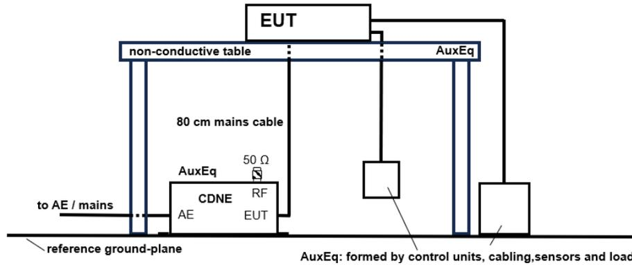
Example of arrangement of an external module during the radiated (OATS, SAC or FAR) disturbance measurement
