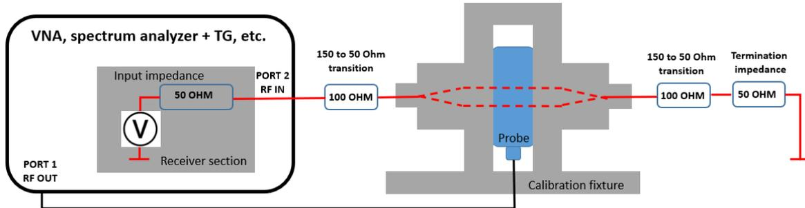
Depending on standard, the BCI-probe may be needed to be characterized in a 300 Ohm loop. Add two 150 Ohm to 50 Ohm adapters and measure S21.
