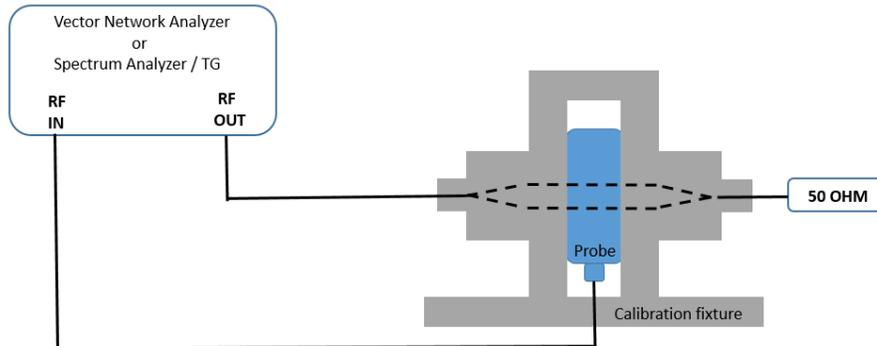
Set the Vector Network Analyzer or Spectrum Analyzer / Tracking Generator to the frequency range of interest and make a through calibration including the two coaxial cables. Connect the RF output to the calibration fixture and the receiver input to the current probe and measure S<sub>21</sub> (insertion loss / coupling).
