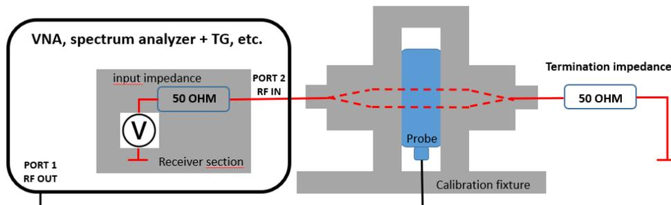
Adding the source impedance of the VNA with the termination impedance of 50 Ohm results in 100 Ohm loop impedance. Measure S<sub>21</sub> to characterize the insertion loss.
