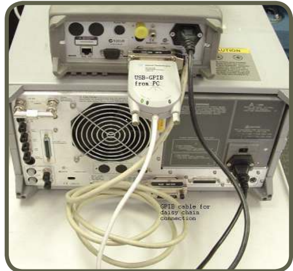
Network Analyzer and Power Meter Setup Showing Power and USB Cables
