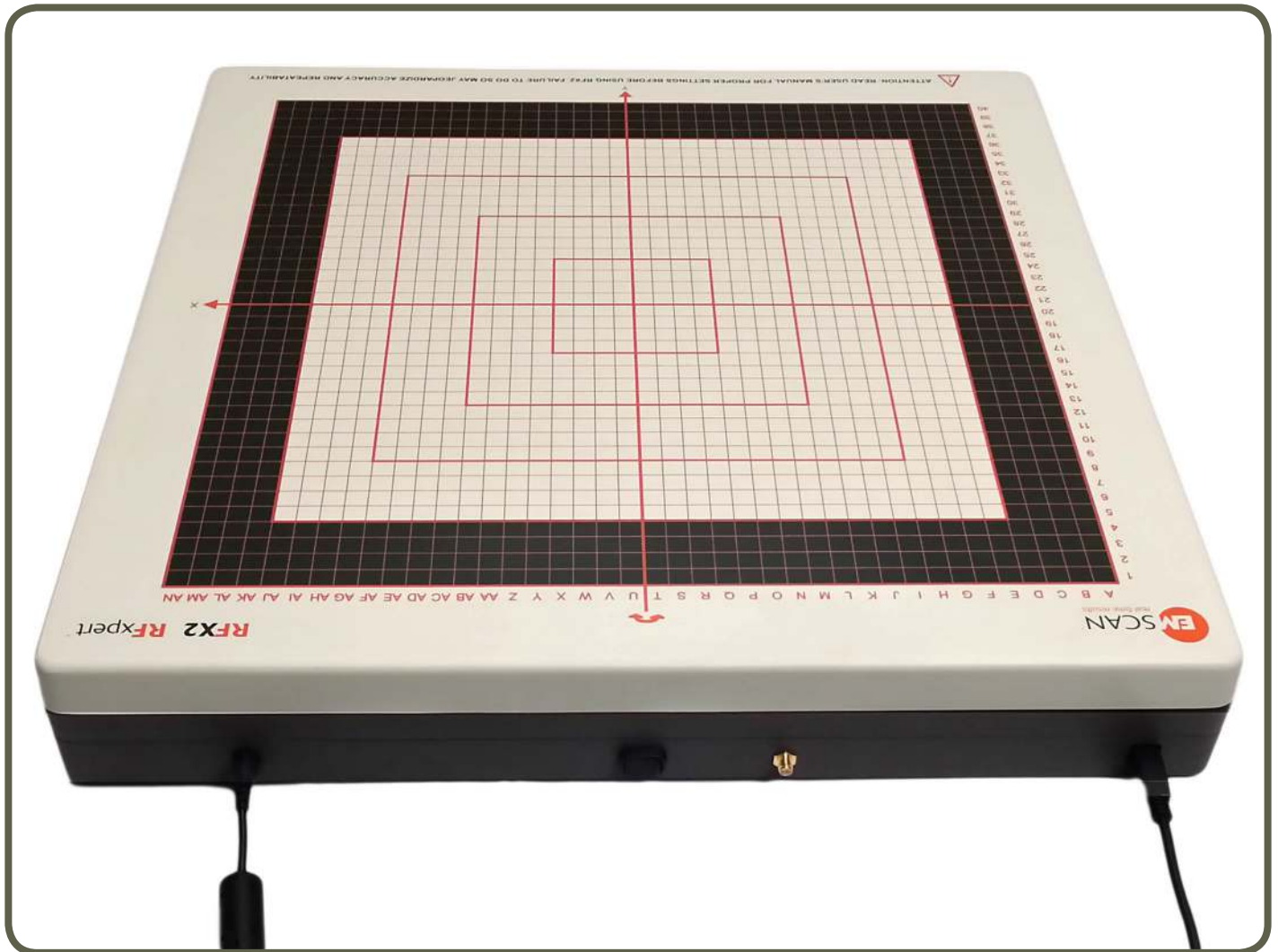
RFExpert Setup Showing Power and USB Cables (RFX2 model shown in the picture)
