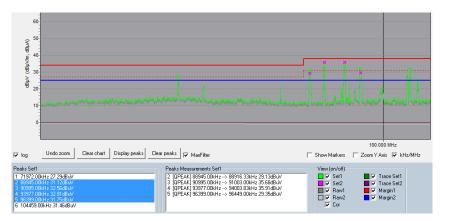
The Peaks Measurements box then displays the results of the fast quasi peak measurement. In addition, the graph shows a cross at the respective frequency and level.
