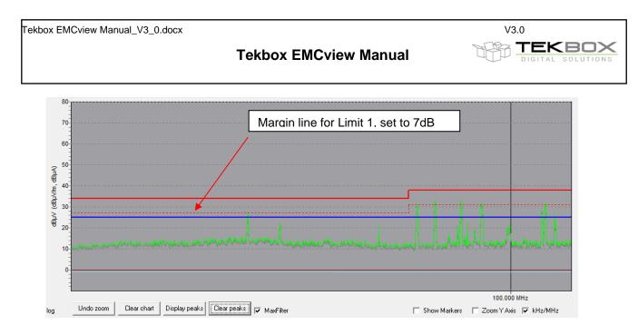
By default, the margins are set to 0, so any peak crossing the limit line would be indicated. Setting margin1 to e.g. 7dB would select all peaks coming within 7 dB close to the limit line of the graph measured with Settings1. Peaks crossing the margin line or limit line can be listed in the in the **Peaks window** by pressing the **Display peaks** button. See chapter 19 on how to manually select peaks and transfer it into the peaks list.
