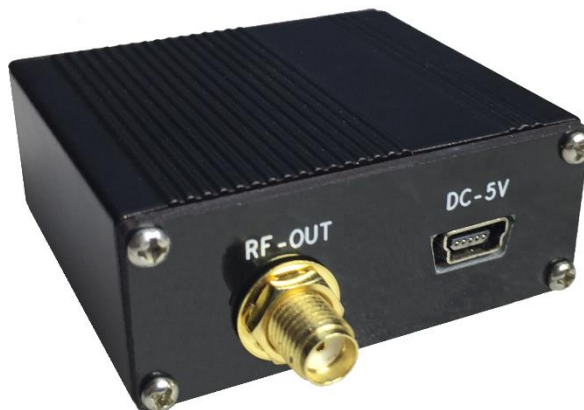
Picture 2 – TBWA2 wideband amplifiers rear view
