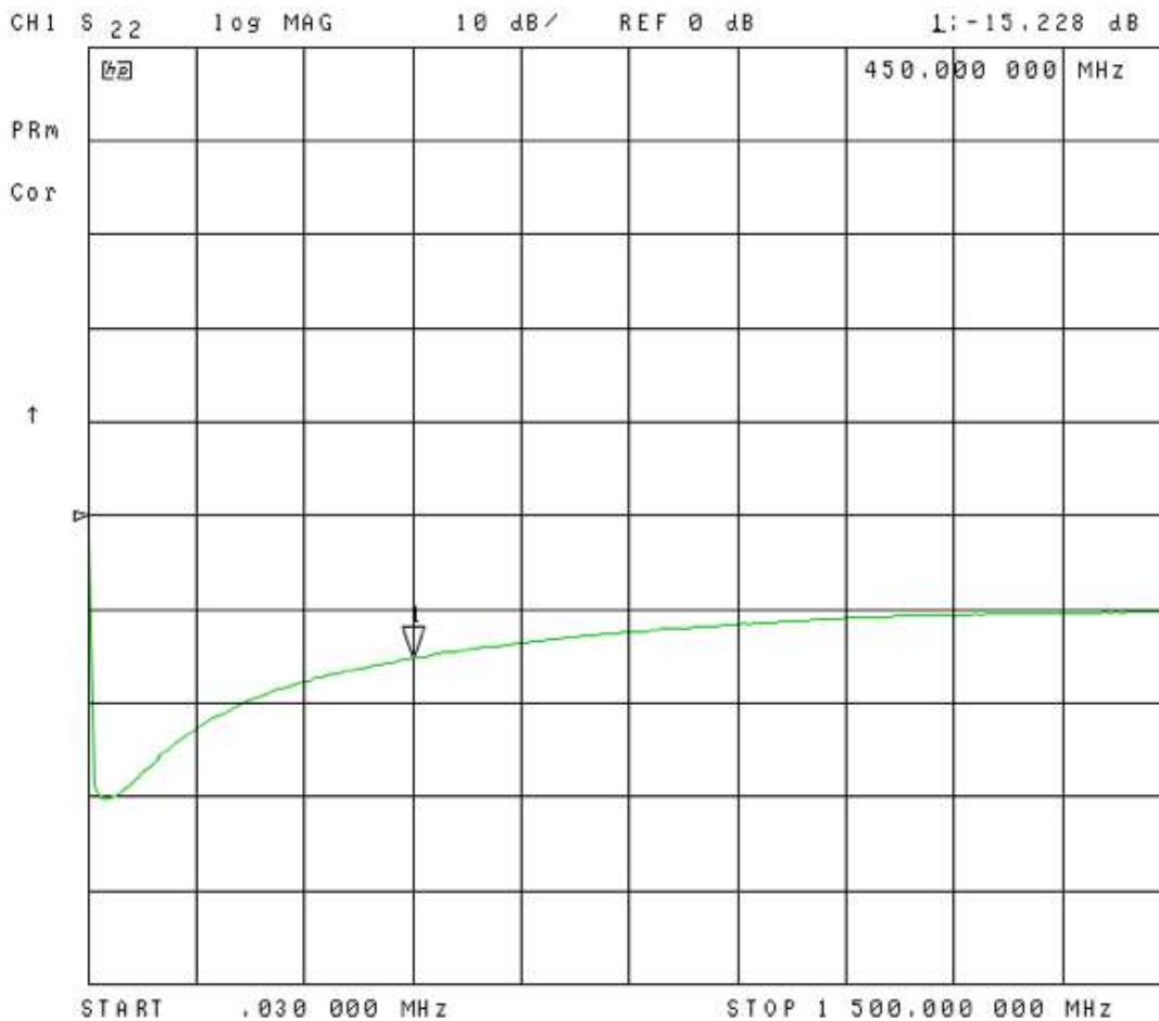
Picture 7 – TBHDR1, output return loss, IS221, 30 kHz – 1.5 GHz
