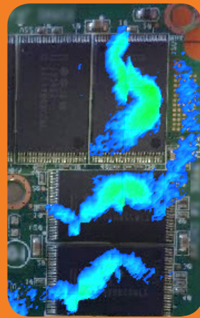
The ERX+ and spatial scan result of a solid state hard drive at 166.028 MHz and 0.12 mm resolution
