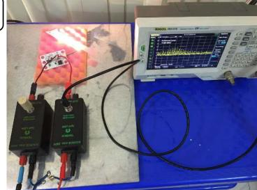
The DUT shall be isolated and elevated from the groundplane. The spectrum analyzer shall measure the conducted emissions on both supply lines. The RF output of the unused LISN shall be terminated with 50 Ohm. In case of a DUT with locally grounded return line, a set up with a single LISN is sufficient.
